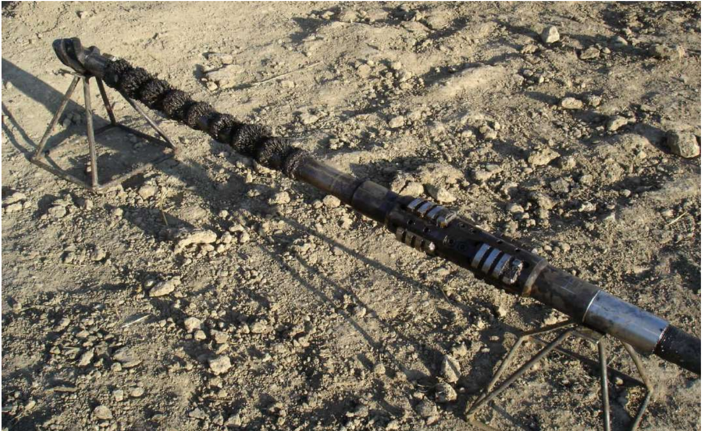
Magnet/Scraper ran after perforating.
